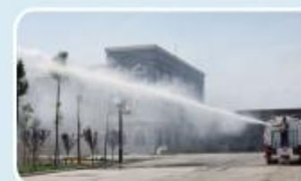
The rear water cannon with a large range can wash high billboards and other places that are inconvenient to clean on a daily basis. The water cannon can also be adjusted to spray mode for long-distance garden spraying operations.
