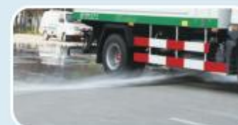
The flushing system can flush road stones, peels and other debris to the roadside. The flushing width can reach more than 24 meters.
